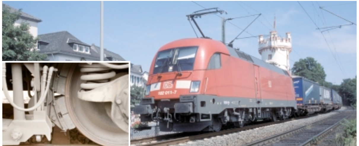
K brake blocks make for smoother running and quieter braking. Photo: DB AG/Pierlings
