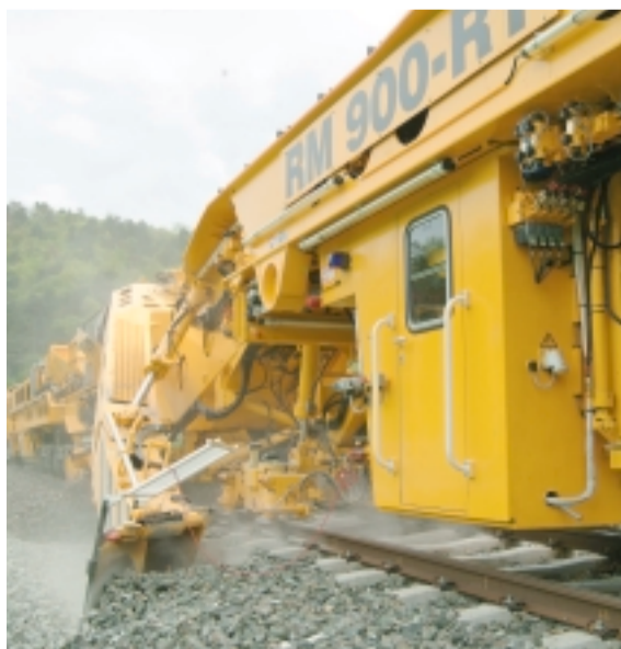
Cleaning output of the HOBCS is up to 400 metres of track per hour
