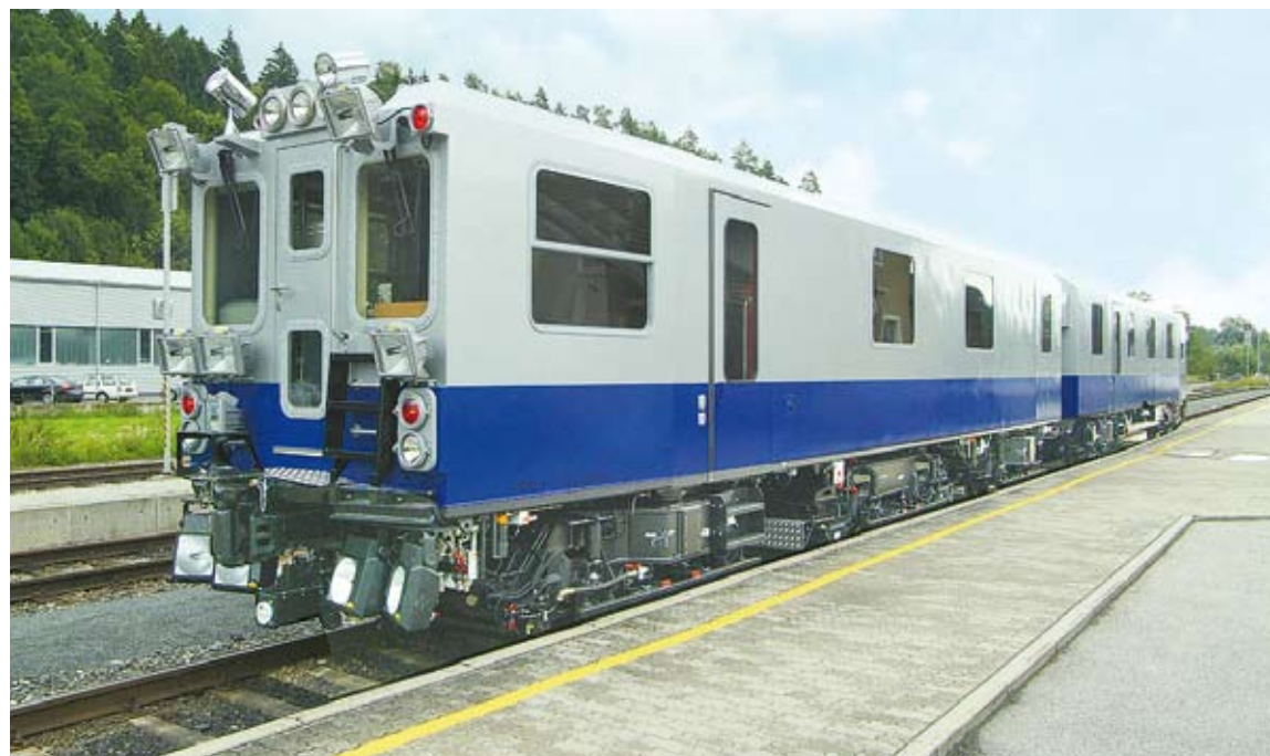
Operating at a speed of up to 160 km/h on the network of Union Pacific Railroad in North America: The high speed universal track recording car EC-5.
