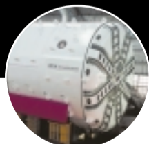
Schluechtern Shield, Closed and Open Mode Ø 10.24 m
