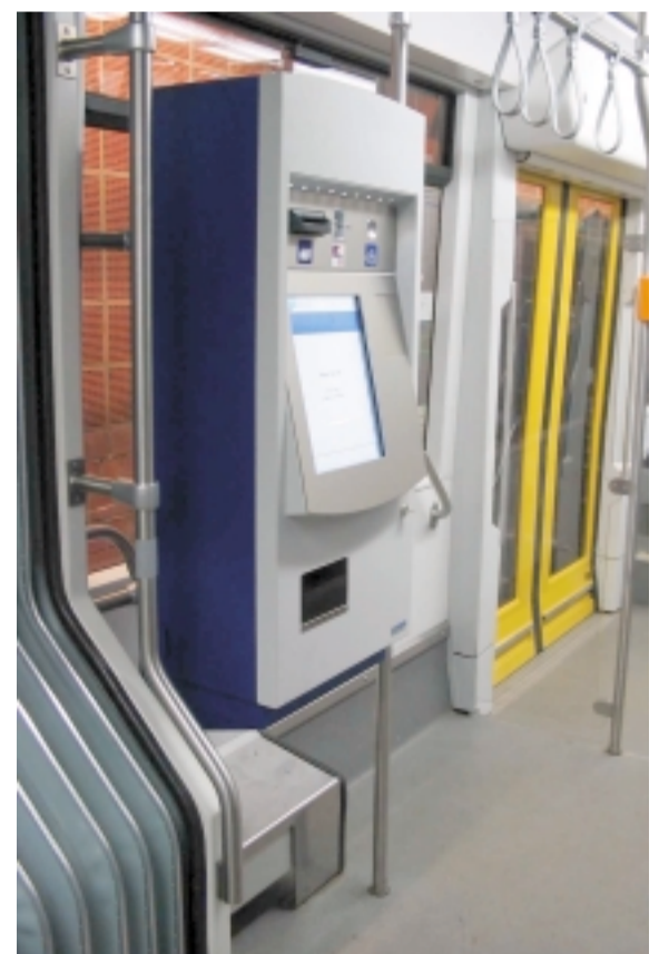
Big displays and touch-screen operation are aimed at ensuring the machines (here on the Kassel public transport system) are easy to use
