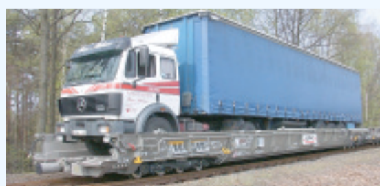
Scheduled for delivery by 2004, the new intermodal low-loader wagons now enable 4 metre high trucks to be carried
