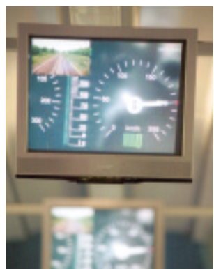
Data from the cab of the locomotive – seen here running at exactly 200 km/h – were relayed to the coaches via monitors.
